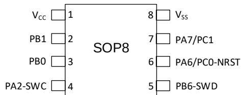
图 3-7 SOP8 Pinout1 PY32F002BL15Sx (Top view)
